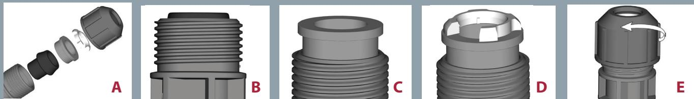
In order to disassemble the Universal nut, follow the Kit assembly instructions in reverse order, keeping in mind that the Universal split ring may require a manual opening of the ends to unfasten the steel grippers from the pipe.
